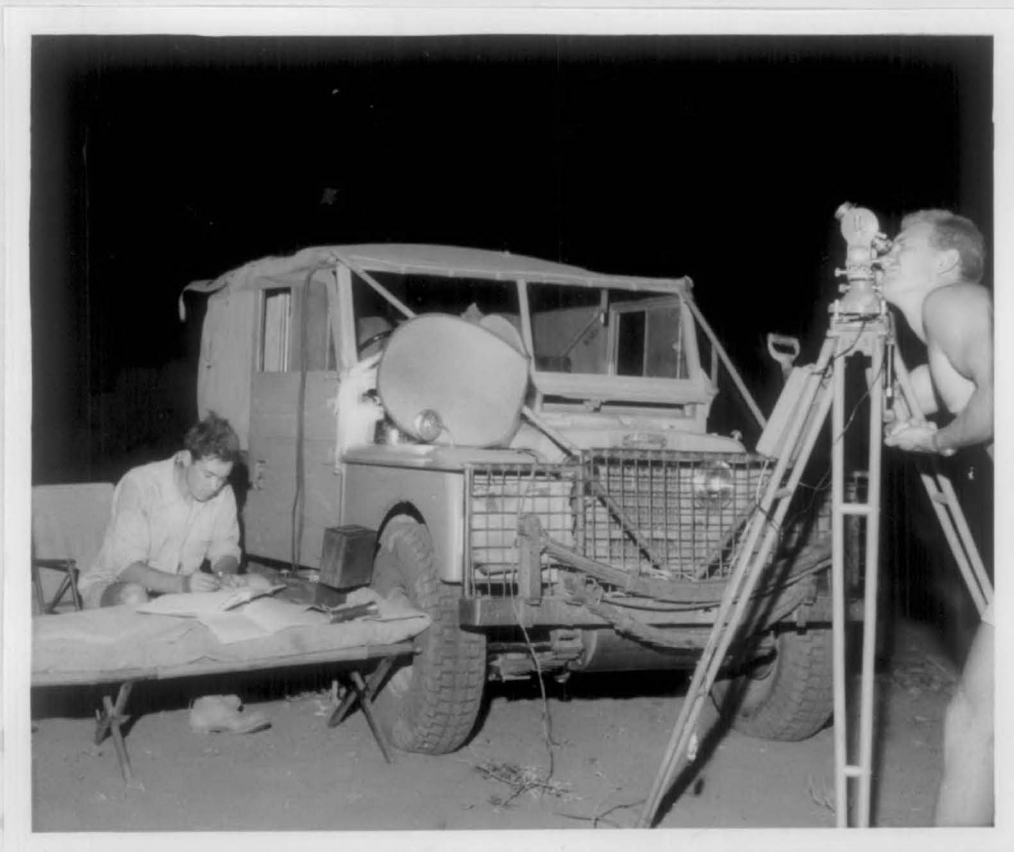
Surveyor Fisher and Geologist Wells observing for Astrofix. Note modifications to vehicles and mounting of spare springs.
