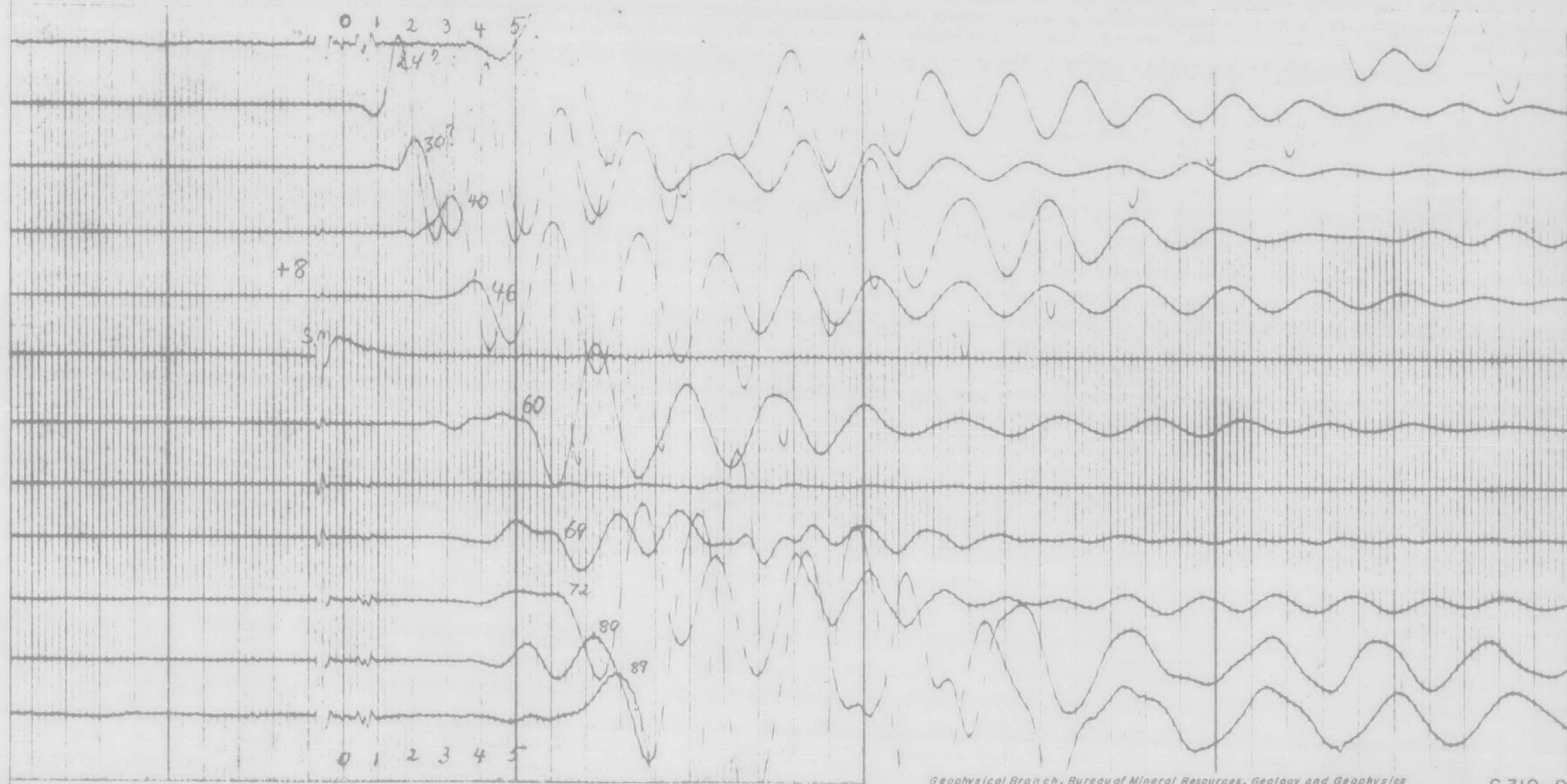
GEOPHYSICAL SURVEY AT THE CLUNY DAMSITE, DERWENT RIVER, TASMANIA FIG.2. SAMPLE OF SEISMIC RECORD OBTAINED DURING THE SURVEY (HORIZONTAL GEOPHONES)
