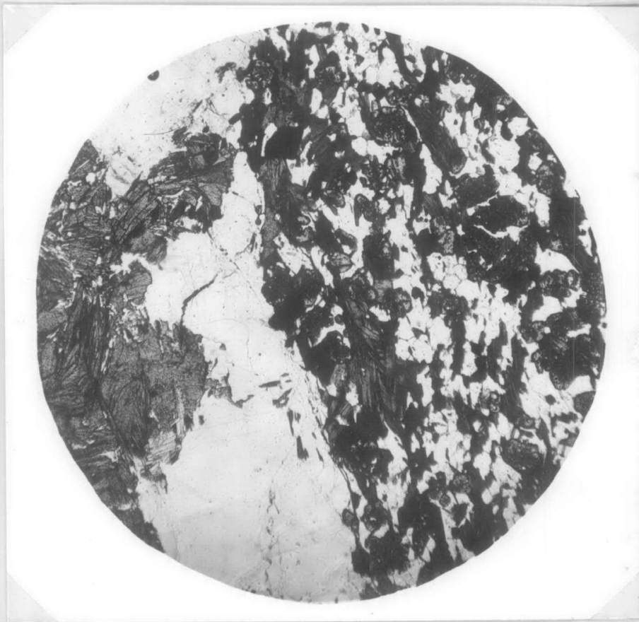
Fig. iii. Specimen 4231: the biotite-garnet-quartz-schist at the right of the photograph is cut by a vein, part of which is shown on the left, consisting of quartz and chlorite. Quartz is white, with low relief: garnet forms subidioblastic grey grains with very high relief. Chlorite is dark grey, and biotite forms very dark grey flakes. Ordinary light X20.
