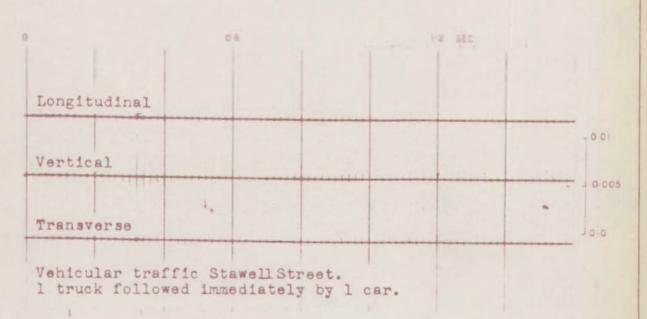
VIBRATION TESTS, GENERAL TELEVISION CORPORATION Pty. Ltd. RICHMOND, VICTORIA, 10/12/59. (Using Sprengnether Vibration Seismograph).
