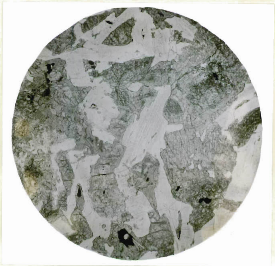
Figure 2: Duchess - Thin section of microgabbro showing feldspar laths, with numerous parallel trains of fine inclusions, ophitically intergrown with partly uralitized pyroxene. Scapolite, biotite, and opaque iron mineral occur in small amounts. (x 27).
