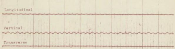
RECORD No2. Compressors A and B running at full load. Recorder on concrete floor 8 feet from compressor A foundation.
