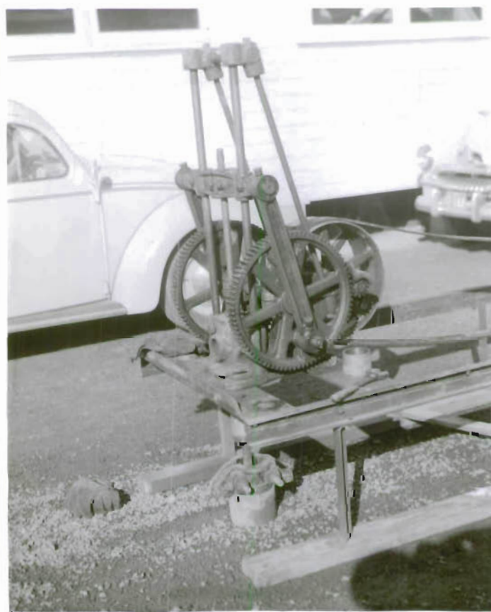
Plate VI: Type A.26, Double-gearred Pumphead with variable stroke for Jack pump.
