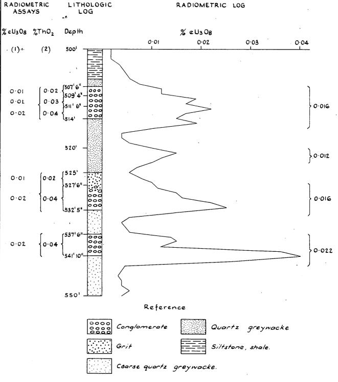
(1) Using U308 (pitchblende) standard. (2) Using ThO2 standard. Thorium responsible for radioactivity measured.
