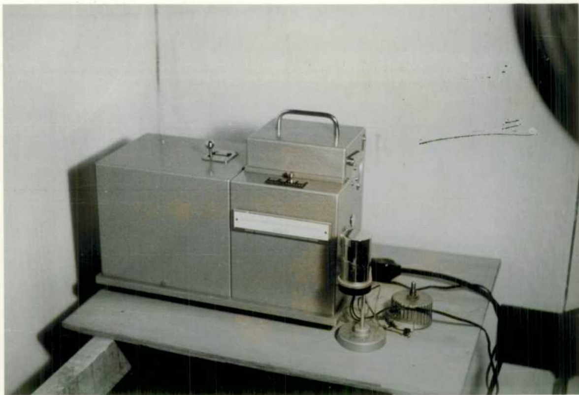
(b) DETAIL OF KIPP RECORDING CAMERA
