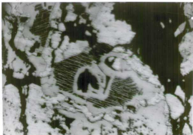
Replacement of a mineral, along the (III) cleavage, by chalcopyrite. The outline of the original mineral is clearly preserved. Chalcopyrite, mid-grey, pyrite-marcasite intergrowth, light grey, calcite gangue, black (X400).
