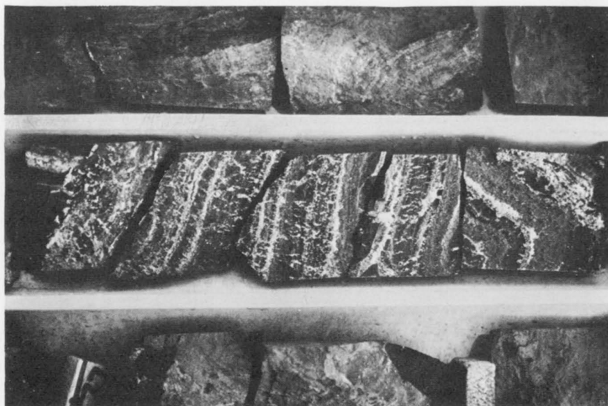
Fig. 12. Chalcopyrite filling tension cracks in crenulated and mineralized shale. HQ core.
