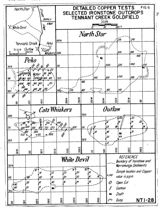
Fig. 6 shows the results of detailed sampling on selected ironstone outcrops in the Tennant Creek Gold ... The tests at Peko, Cat's Whiskers, and Outlaw were primarily carried out to check the reliability of 50 foot spacing of sampling along the trend of the ironstone outcrops. The North Star and White Devil tests were added because the extension of these bodies at depth had been tested by drilling.
