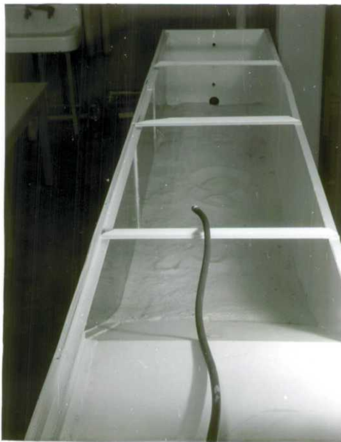
Fig.2. Sand is hosed into tank from shelf in foreground. Water level in tank controlled by valve outlets in far end of tank (one outlet is hidden by bar).
