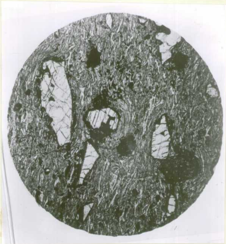
Figure 3. Dacite ignimbrite of the first volcanic epoch. Note compacted and welded glass shards of groundmass. Phenocrysts mainly plagioclase (cleaved), some embayed quartz, some augite and iron ore. X35, ordinary light.
