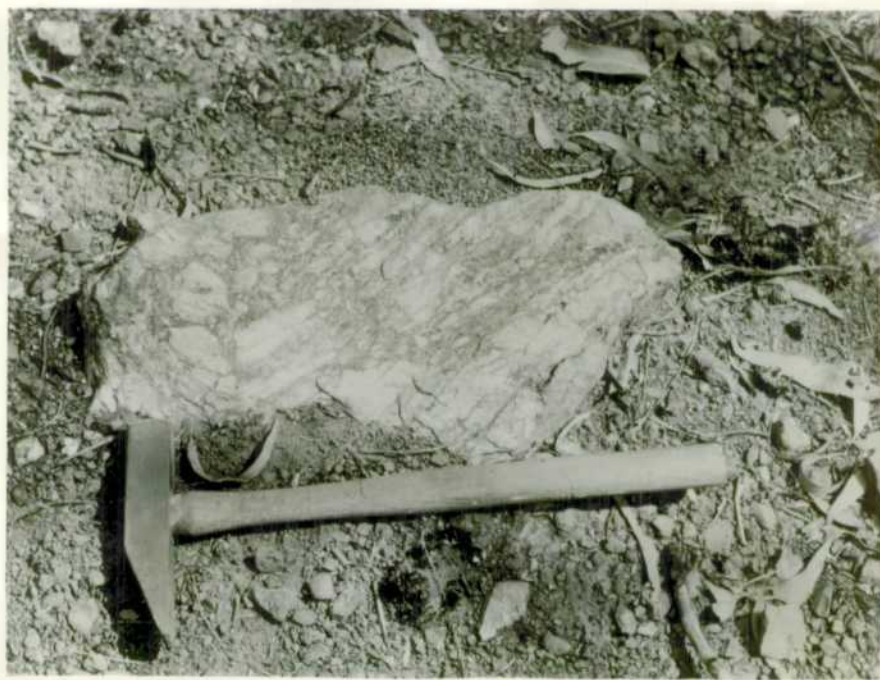
Figure 1. Minor fold in quartzite breccia. Matrix is hematite.
