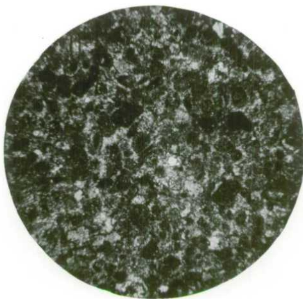
Figure 1 : Mail Change Limestone: buff-grey mottled calcilutite in outcrop. Contains pellets, shell fragments and algal filaments in thin section. Mottling is due to dolomite rhombs. Photomicrograph shows small pellets in a fine-grained calcite matrix.
