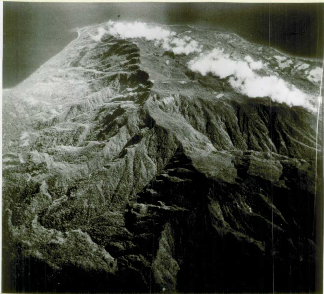
Figure 23. Northerly-plunging anticline forming the Oiatabu Range on Fergusson Island. Some dip slopes are visible on the flanks of the range.
