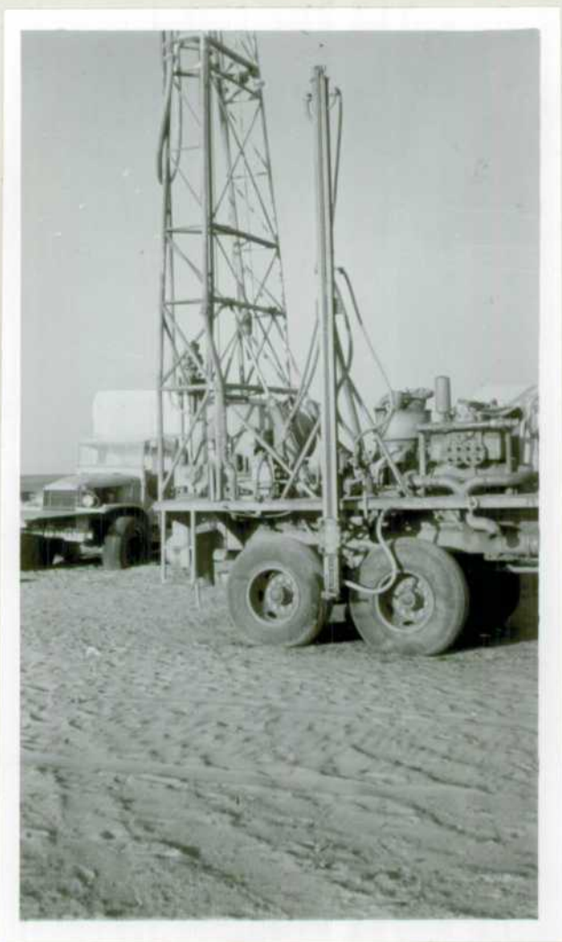
Figure 8 Wagon Jack percussion drill mounted on the side of a Faling 1500 rig truck
