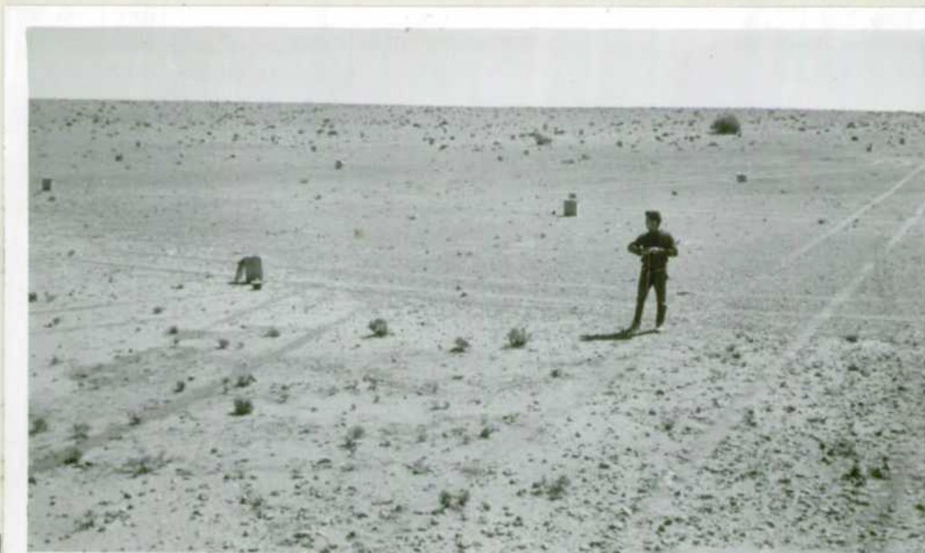
Figure 4 Preparing a surface pattern shot for refraction shooting.
