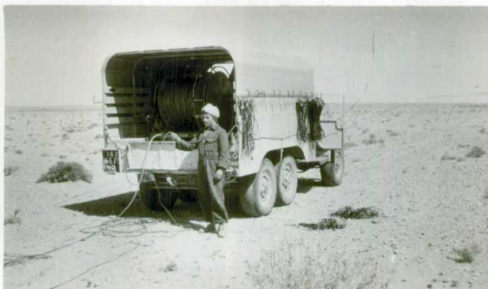
Figure 7 Cable truck on CGG refraction party, showing heavy geophone cable on power driven reel.
