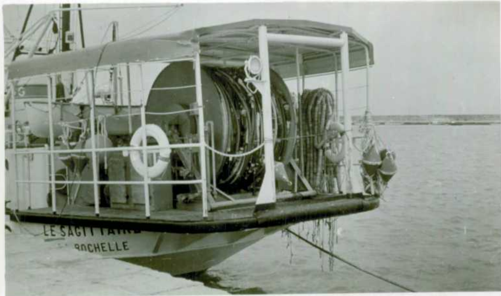
Figure 12 Marine seismic cable at stern of CGG recorder boat, Sicily
