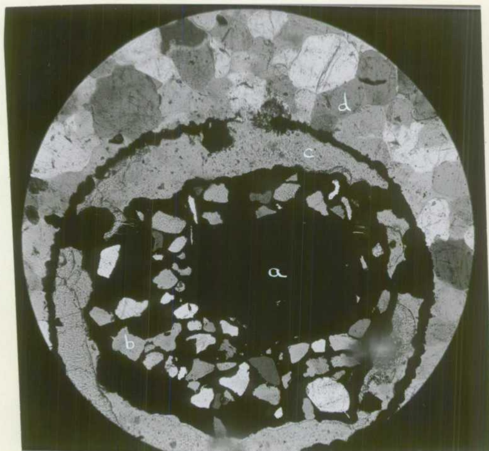
Fig. 24. Thin section of coarse grained sandstone with vughs. Pacoota Sandstone.
