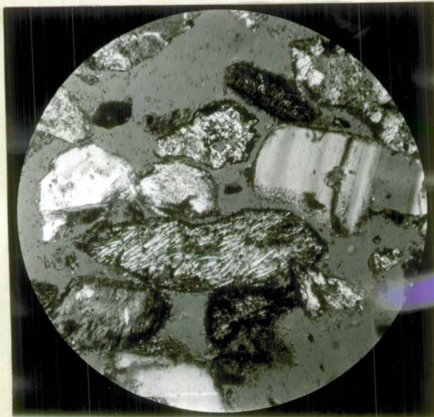
Fig. 7. GAB 847. Lithic-feldspathic sandstone, showing grain of andesite near centre, plagioclase near right edge. Crossed nicols, X140
