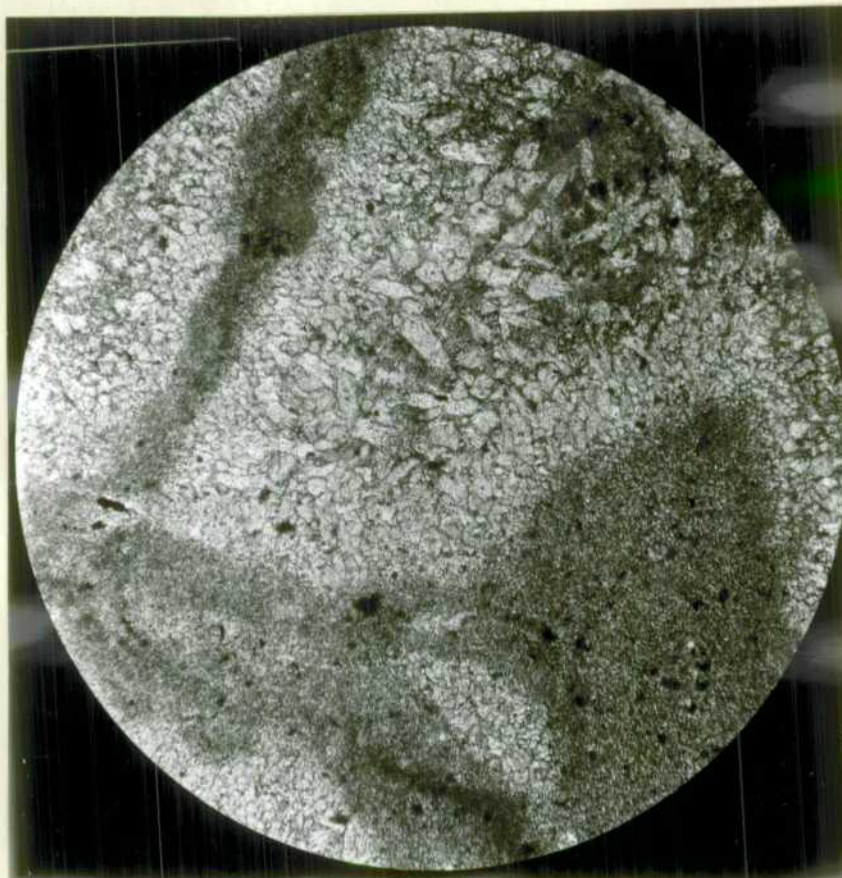
Fig. 4. GAB 1017C. Calcite replacing clay in brecciated limestone. Calcite crystals originate from veinlets of microcrystalline calcite; note radiating crystal growth in upper right. Ordinary light, X60.
