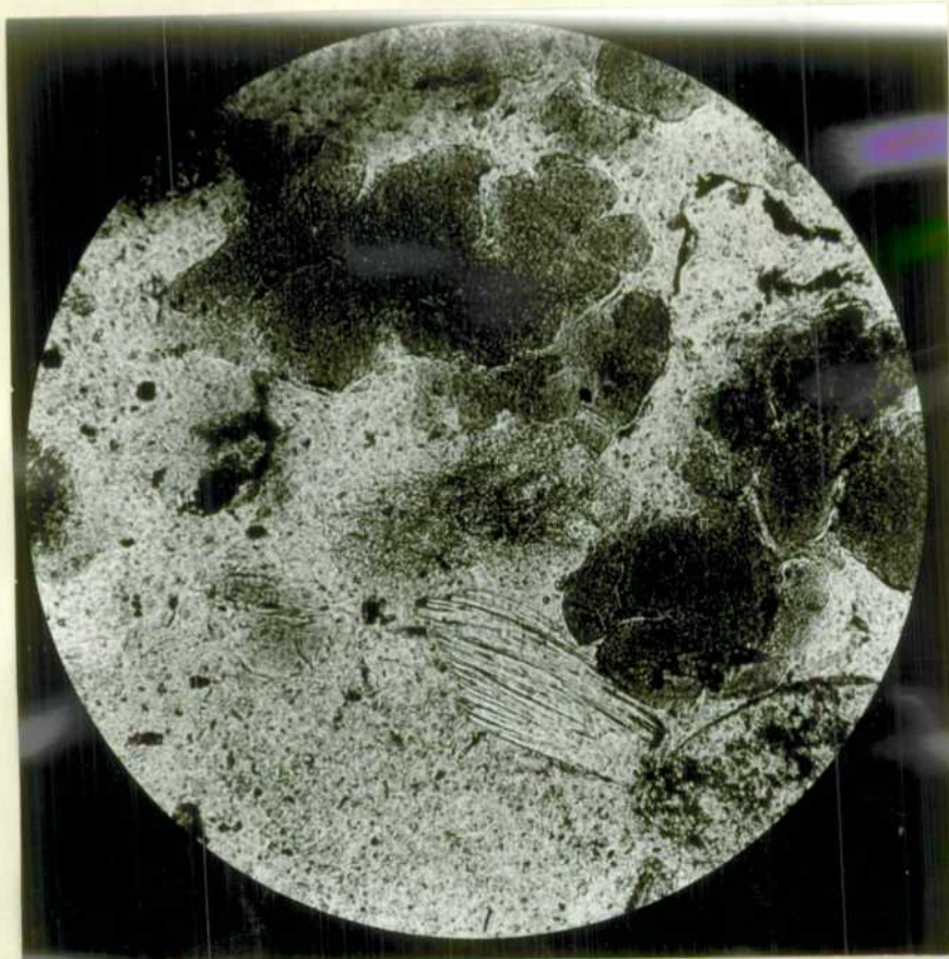
Fig. 2. GAB 1017E. Grains of glauconite in silty clay, with a grain of muscovite expanded slightly by alteration to glauconite along its cleavages. Ordinary light, X210.
