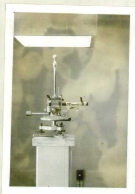
Ruska Magnetometer (note method of illumination)
