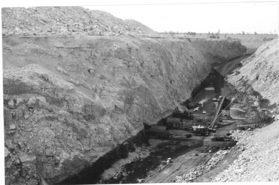
Figure 14: Thiess-Peabody's Moura open-cut. The coal dips westerly, and the overburden consists of hard feldspathic sandstone. (Neg. No. M/323).
