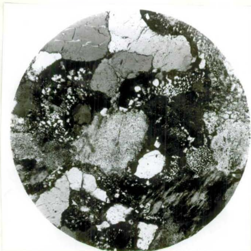
Fig. x: Specimen R.14152 from the xenolithic dyke southwest of Mt Mulligan. An early stage in the fusion of a xenolith. Micrographic material may be seen on crystal boundaries. Crossed nicols, X55. B.M.R. Negative No.G4991.
