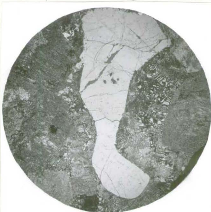
Fig. xi: Specimen R.14155 from the xenolithic dyke southwest of Mt Mulligan. A later stage in the fusion of a xenolith. Feldspar (dark grey, top and bottom of the photograph) almost entirely separated from quartz (very pale grey to white, photograph centre) by granophyric material. Note the embayed and corroded form of the quartz. Crossed nicols X20. B.M.R. Negative No.G/4992.
