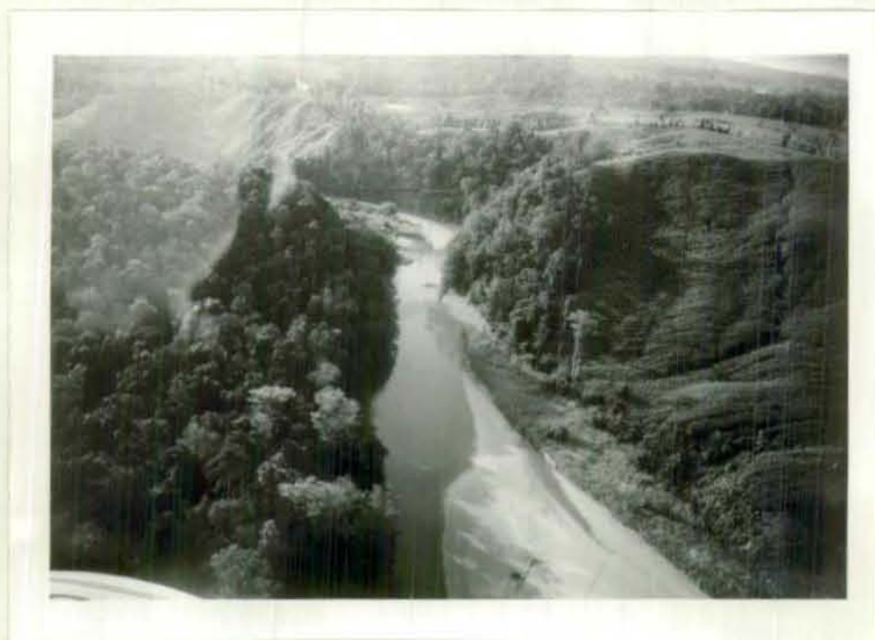
Figure 1: Left abutment of Damsite A - volcanic agglomerate with jointed basaltic dyke near left hand of photograph.
