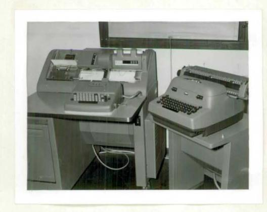
Figure 45: The 870 Document-Writing System. The instrument on the left is the 836 card-punch, card-read machine; that on the right is the 866 automatic type-writer.
