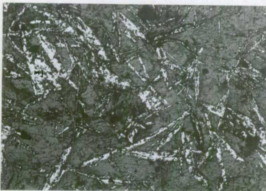
Fig. 15. Foliae of magnetite (mg) scattered through a talc gangue.
