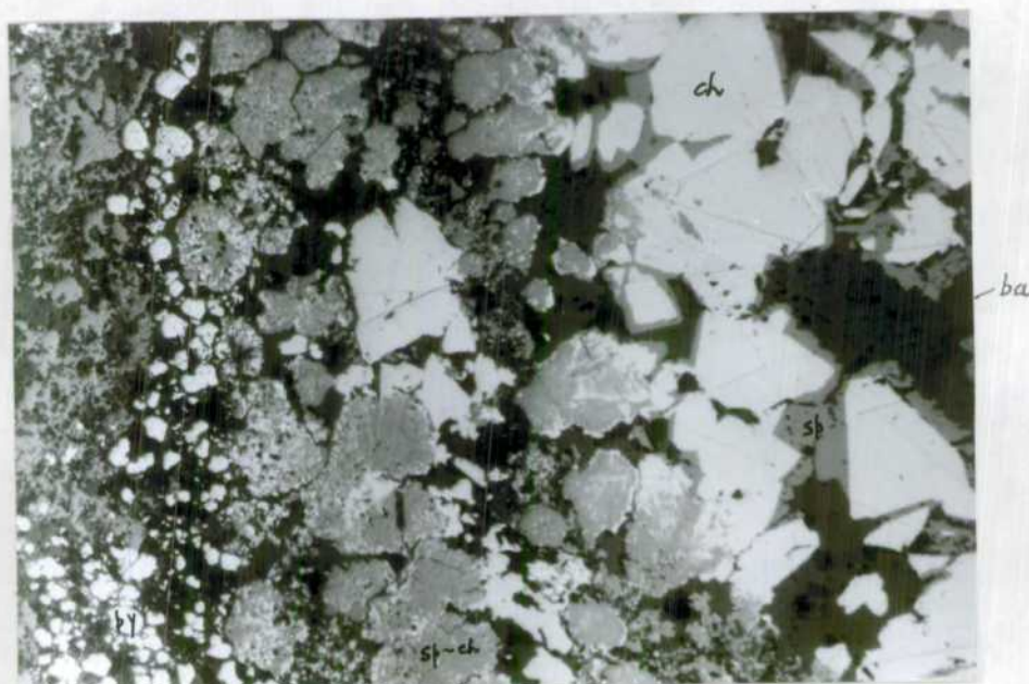
Fig. 2. Banding of sulphides. Right hand band contains chalcopyrite (ch), surrounded by sphalerite (sp), in a barytes gangue (ba). In the centre band sphalerite is partly segregated from chalcopyrite (sp-ch). The white grains in a band on the left hand margin are subhedral and spheroidal pyrite (py).
