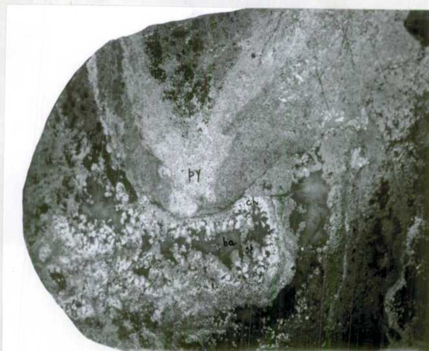
Fig. 1 Banding and folding in sulphide ore. Chalcopyrite (ch), sphalerite (sp), fine grained sub-hedral and spheroidal pyrite bands (py), barytes gangue (ba). Figs. 2-9 are from areas in the main fold.
