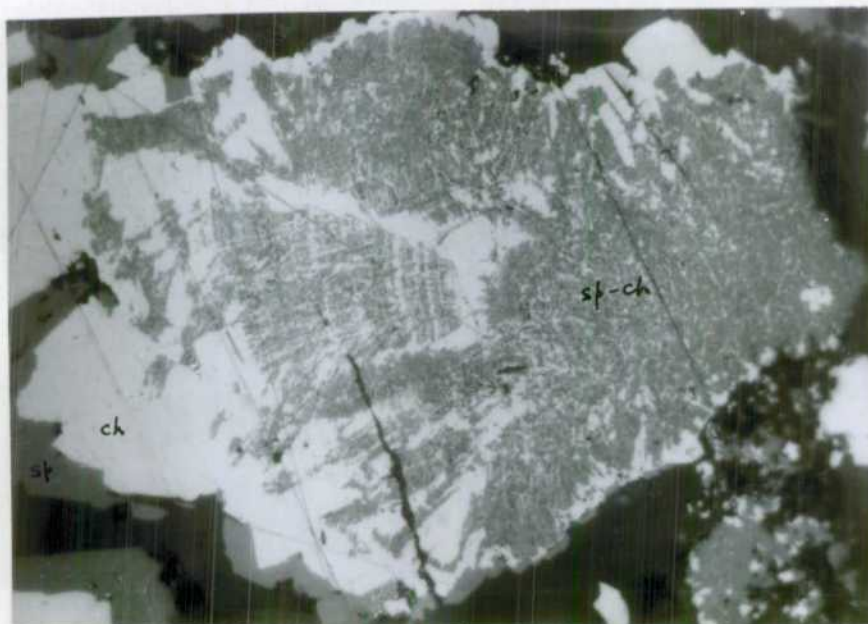
Fig. 8. Textures indicating segregation of sphalerite (sp) from chalcopyrite (ch) and forming rims around chalcopyrite.
