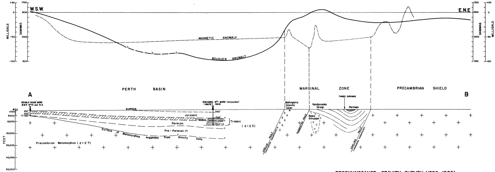
The stratigraphy was suggested before the completion of ENEABBA bore Triassic beds proved to be much thicker than expected and the metamorphic basement may be much deeper than shown
