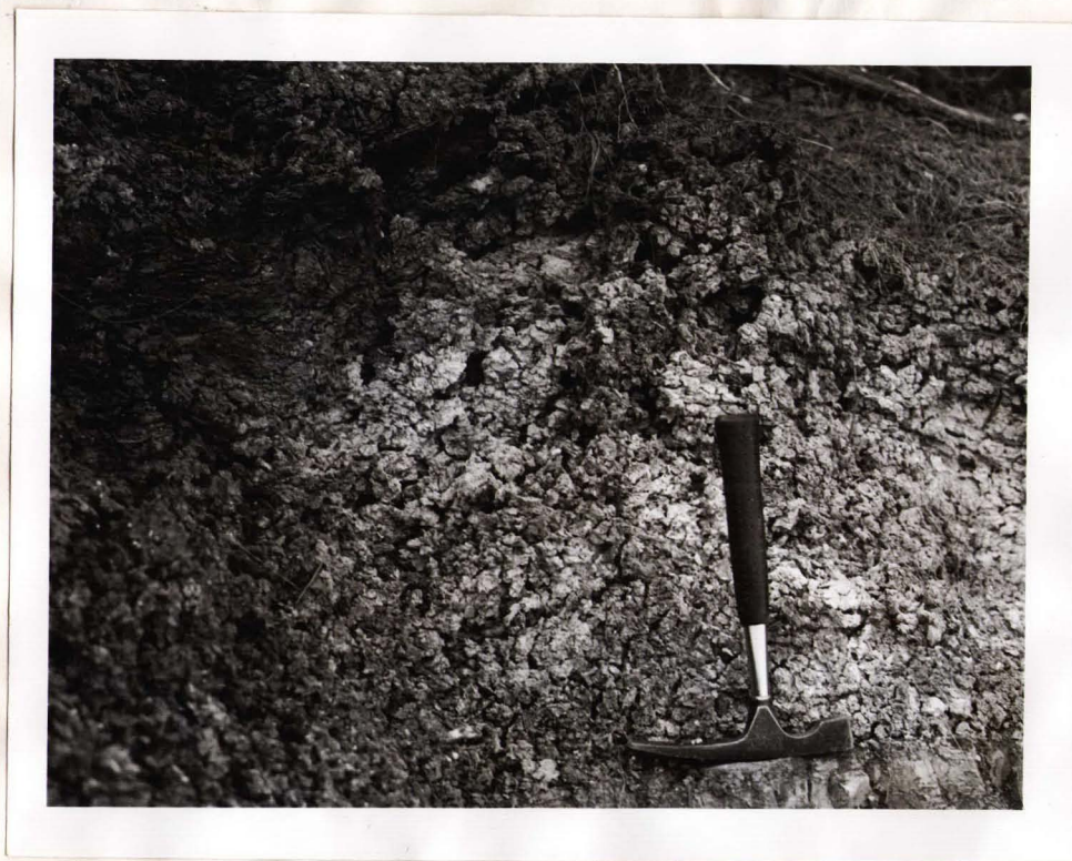
Figure 3 : Swelling bentonite exposure at site of sample E \frac{1}{4} mile north-east of Early Storms homestead.
