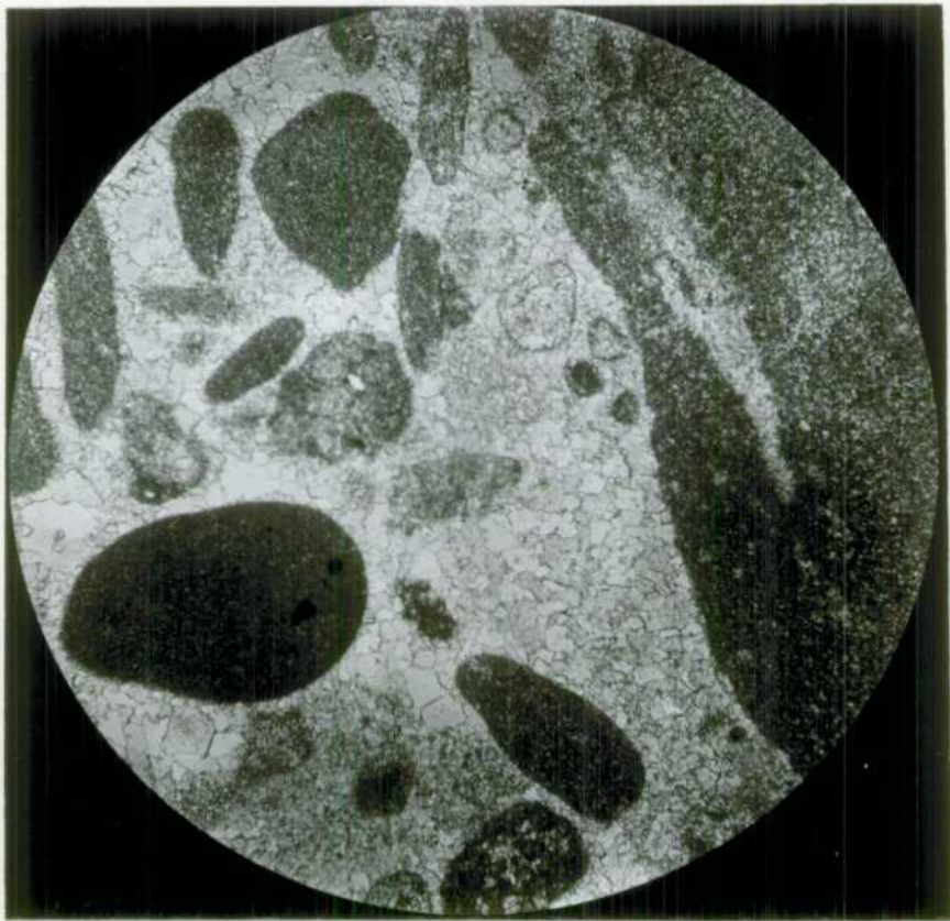
Fig. 5. Meeta Beds , showing dolomitic intra-sparudite, with clasts of micro-crystalline dolomite in dolomite cement (left) and partly recrystallised micro-crystalline dolomite. X30, (SR 266), File No. g/8259.
