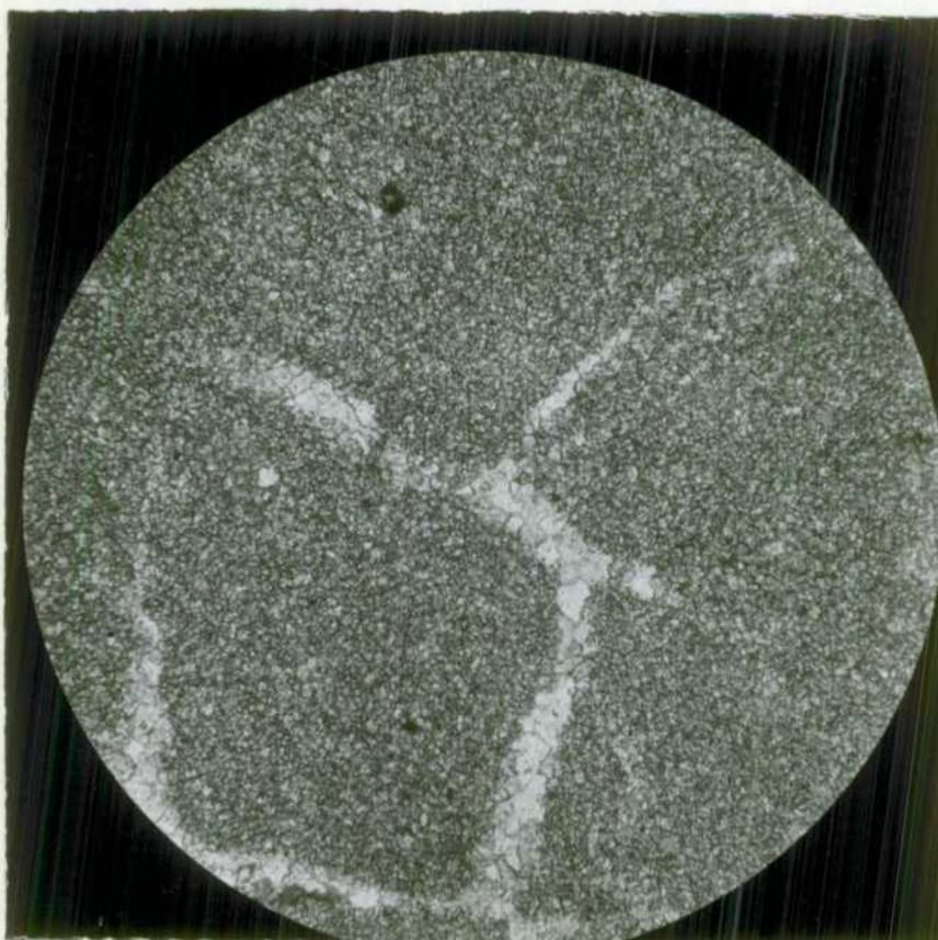
Fig. 7. Meeta Beds , showing microcrystalline dolomite (dololomite? or primary dolomite?), and veining. X30, (SR 267), File No. g/8265.
