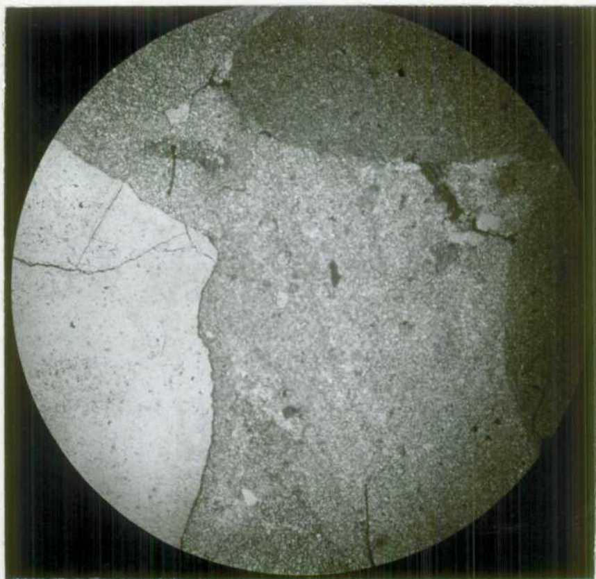
Fig. 3. Meeta Beds , showing dolomitic intramicrudite with large clasts of microcrystalline dolomite (right) and angular chert grain (left) in matrix of microcrystalline dolomite. X15 (SR 253(c)). File No. g/8264.
