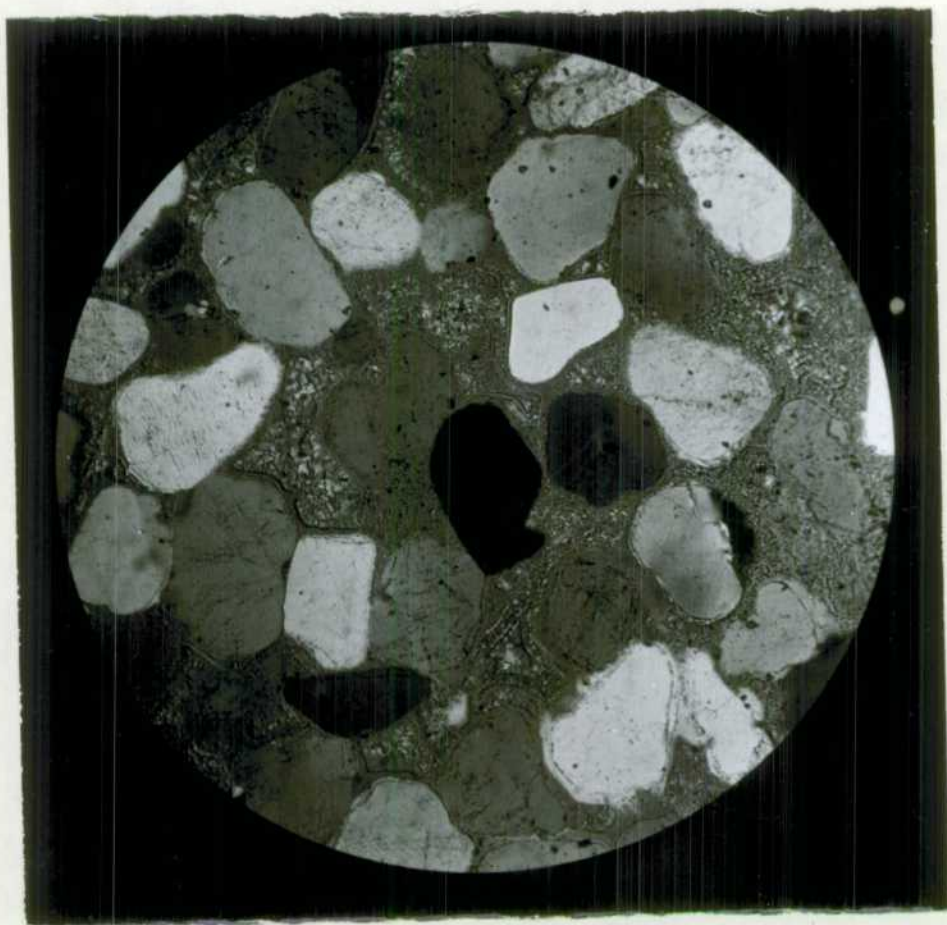
Fig. 18. Meeta Beds showing well sorted siliceous quartz sandstone with fibrous chalcedony veins and drusy siliceous cement. X45 (SR 294 b), File No. g/8192. (x-nicols).
