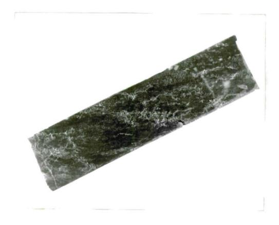
Figure 1. Section of mineralized drill core, D.D.H.1(b), Explorer 17. Post-tectonic chalcopyrite and pyrite (light grey) replacing sheared chloritic breccia matrix (black) along shear planes and between grains of pre-tectonic caraclastic magnetite (dark grey). x2 magnification.
