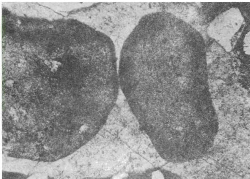
Fig.56 Spec.AP1/97/1 linear mag x 150 Structureless phosphatic pellet with a prominent dark rim - calcareous cement
