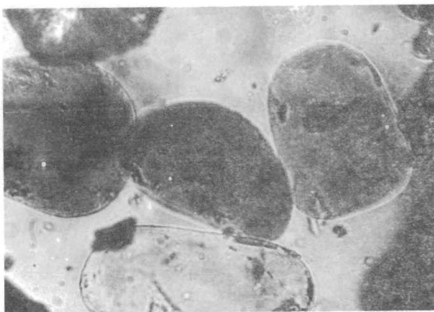
Fig.52 Spec.AP1/628/6 linear mag x 400 Typical super-mature tourmaline - extremely well rounded.
