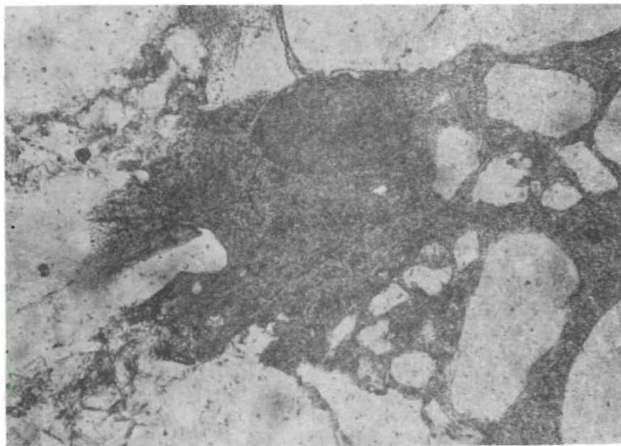
Fig.77 Spec.AP1/51/2 linear mag x 80 Phosphatic pellet (dark grey) with an included glauconite grain (black showing a very sharp margin.
