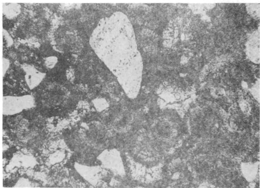
Fig.72 Spec.HY 762 linear mag x 150 Secondary corkite (dark oolitic form) with ?apatite cement (light, high relief). Some quartz grains (white).
