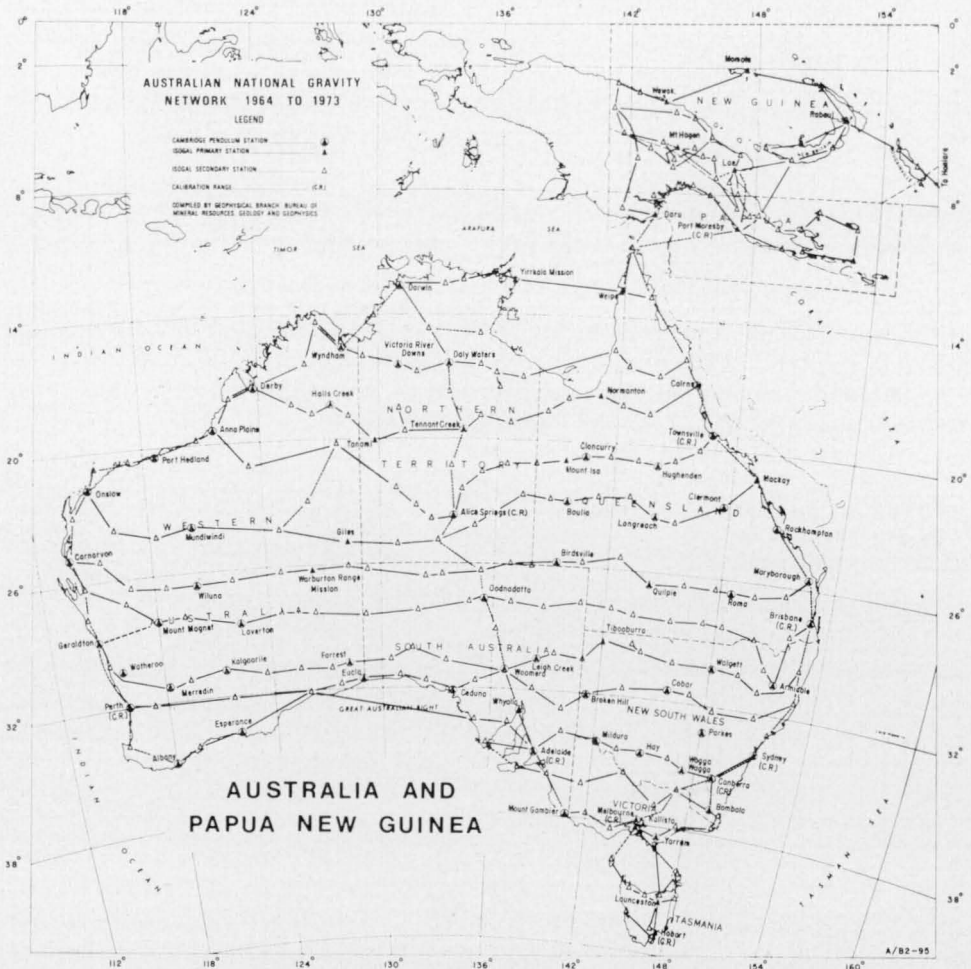
Fig. 2. The Australian National Gravity Network (Isogal Network). The lines of almost equal gravity (solid lines) are joined by calibration lines and tie lines (broken lines).
