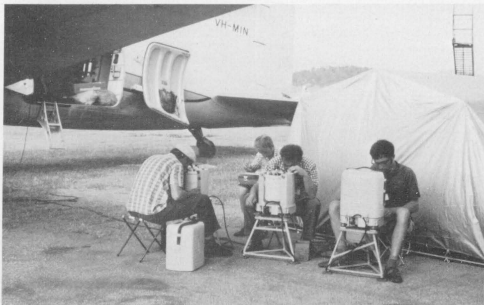
Fig. 6b. Observations being made with GAG-2 gravity meters. Normally the tent shelters the gravity meters.
