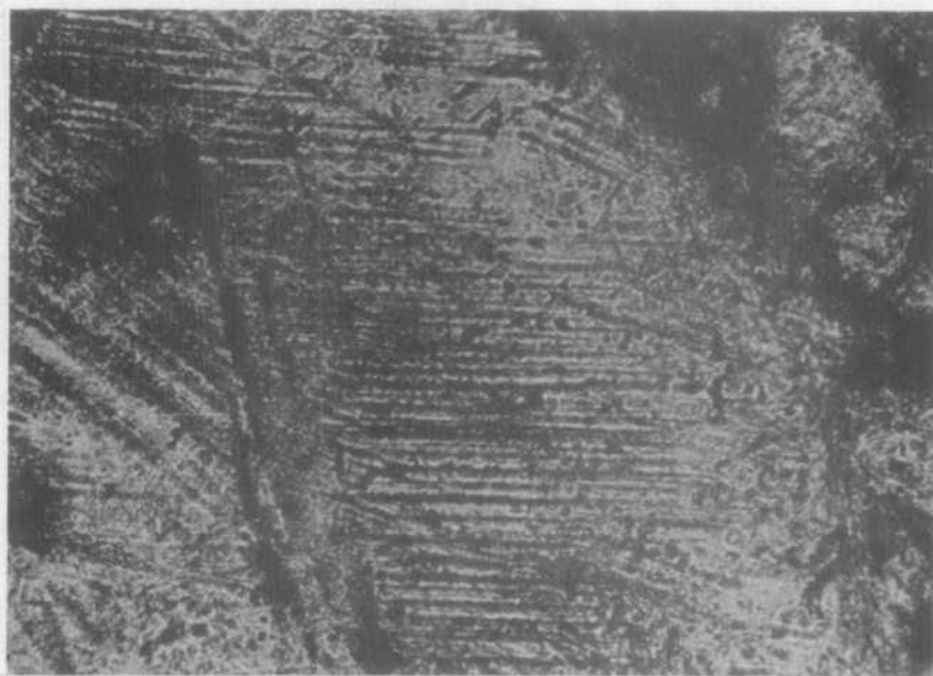
FIG.12 Strain lamellae on the surface of a quartz grain from the Stairway Sandstone equivalent (Ol(1)) present in the centre of Gosses Bluff.
