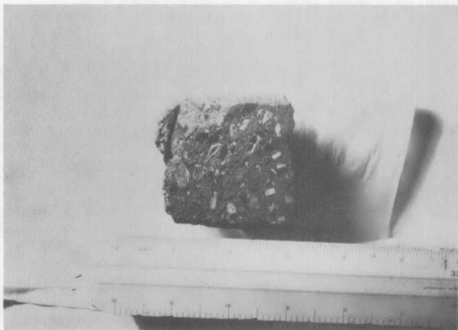
FIG.19 Specimen of breccia with clasts of sandstone, siltstone and claystone. Many of the light patches are composed of bentonitic clay. Specimen from Hermannsburg (B.M.R.) No.5, depth of 27 feet. Scale is marked in inches.
