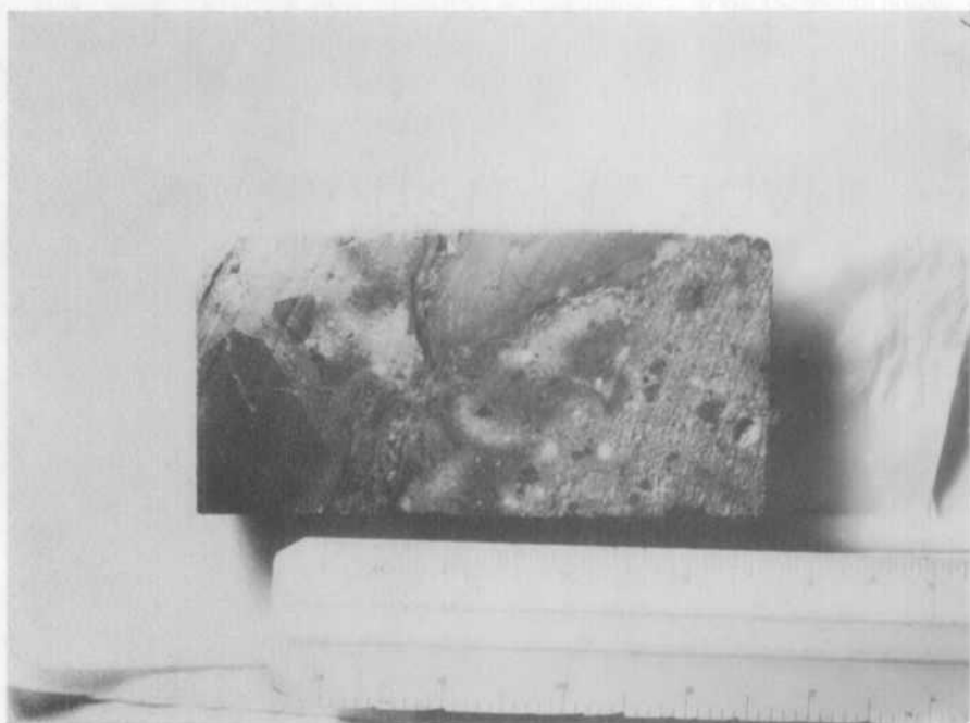
FIG.20 Breccia with extremely angular fragments of sandstone, siltstone and mudstone. In the middle of the core is a lens of bentonitic clay, with an irregular crenulated boundary. Specimen from Hermannsburg (B.M.R.) No.1, depth of 97 feet. Scale is marked in inches.
