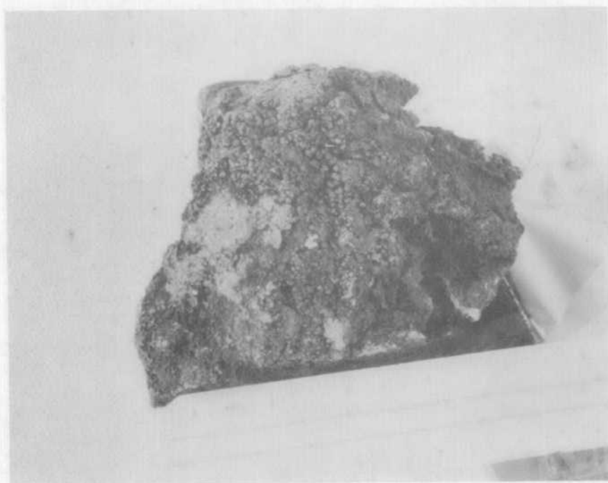
Fig.13 Specimen of glassy zeolitic rock with rounded granules which possibly represent moulds of vesicles in the originally molten rock (?). The specimen is from the eastern peak of Mount Pyroclast. Scale is marked in inches.
