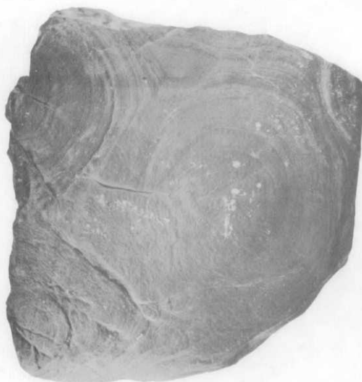
Fig. 2 Algal-stromatolite dolomite, laterally-linked columns, plan view. Meeta Beds, Sandover River area. x\frac{3}{4} (File No. g/5420)
