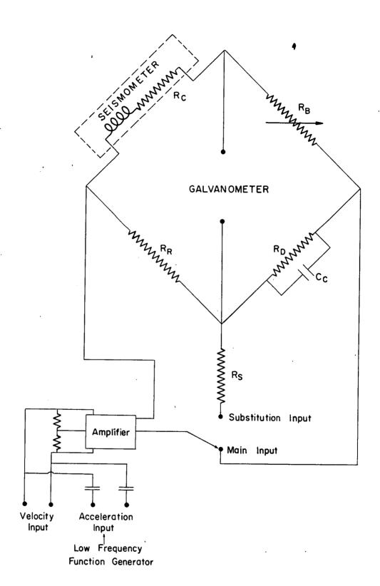
CIRCUIT DIAGRAM FOR WILLMORE BRIDGE METHOD OF CALIBRATION
