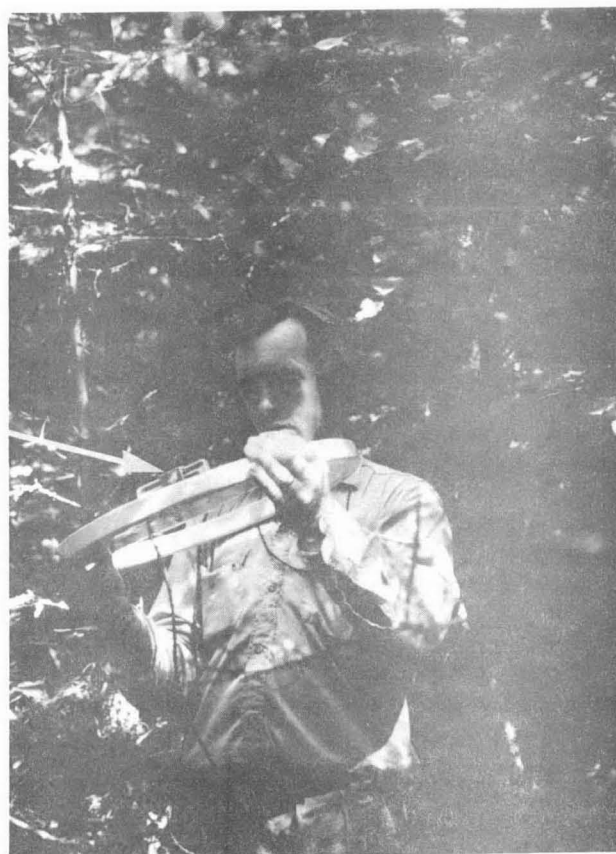
PLATE 9 VERTICAL LOOP EM RECEIVER TAKING DIP ANGLE MEASUREMENT, NEAR TIMMINS, ONTARIO
