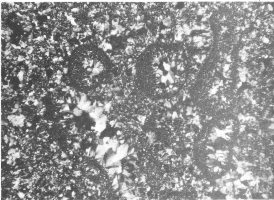
Figure 20: Completely silicified coquinite from 'unnamed chert rubble horizon' 8 miles south-east of Duchess. Crossed nicols to show up ghosts of former skeletal debris. X35
