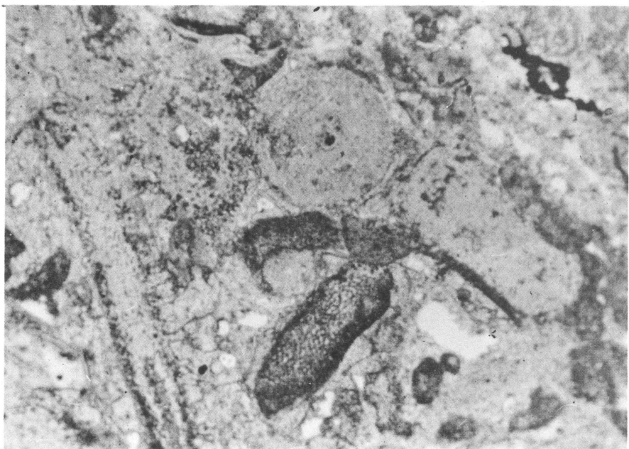
Figure 59: Phosphatic biopelsparite (encrinite limestone). Cystoid and other fossil fragments and some phosphate pellets. Ordinary light. Area 2 miles north of Mount Murray. X35
