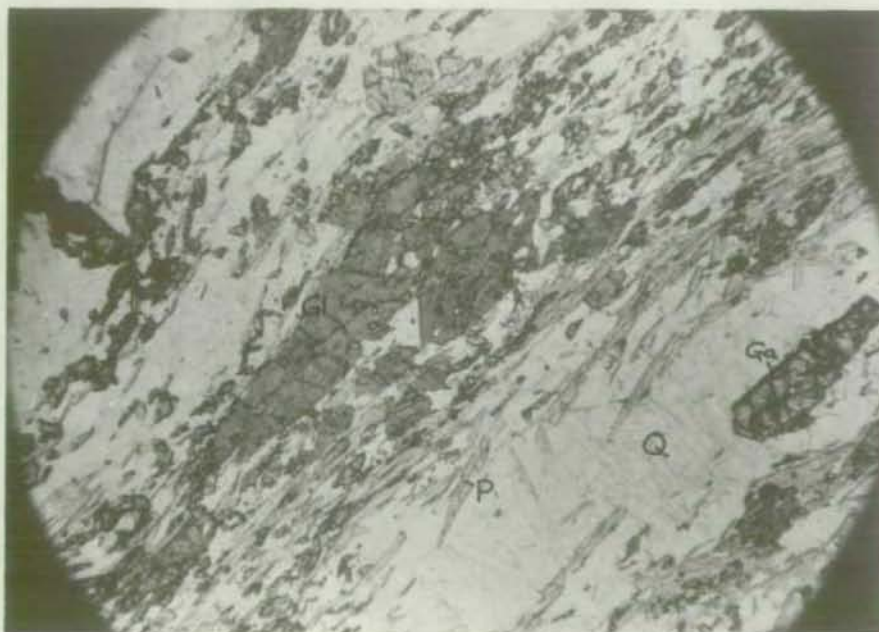
Figure 27B. Quartz, glaucophane, epidote, garnet paragonite schist. 03NG0505 Fl. C Glaucophane (Gl) Paragonite (P) Quartz (Q) Garnet (Ga) Magnification X 35.
