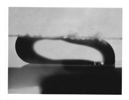
Figure 1: Enlarged photograph showing a droplet of native oil between two crystals of silica in a simulated formation water environment. The crystals are moved vertically together until the drop becomes elongated; one crystal is then displaced parallel to the other in a horizontal plane to achieve maximum distortion of the oil droplet. The contact angle of the oil with the crystal is measured directly on the photo. (Scale approximately 10X).
