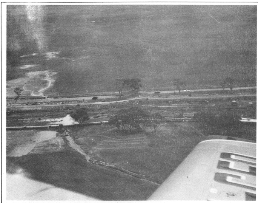
FRACTURE ZONE: (a) Railway cut 1½ miles west of Meckering, looking north. Railway shortening 7 feet. East side up. Pipeline break not visible. (note trees still upright)
