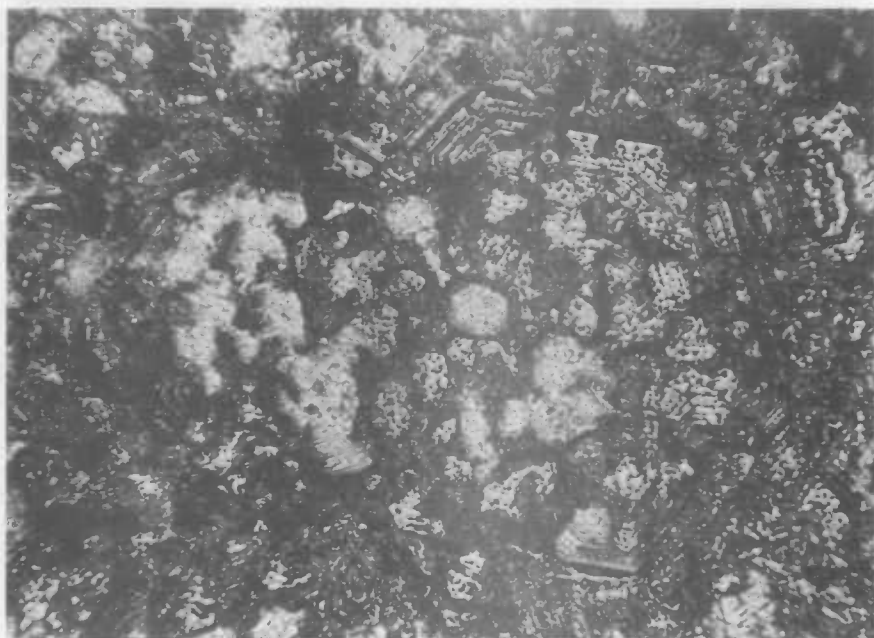
Figure 46: Zoned variscite, meta-variscite, and possibly other Fe-Al-phosphate minerals, forming replacement complex. Original pelletal structure of the rock is still clearly visible in this example. See also Figures 47-49. Photomicrograph, ordinary light. x 60.
