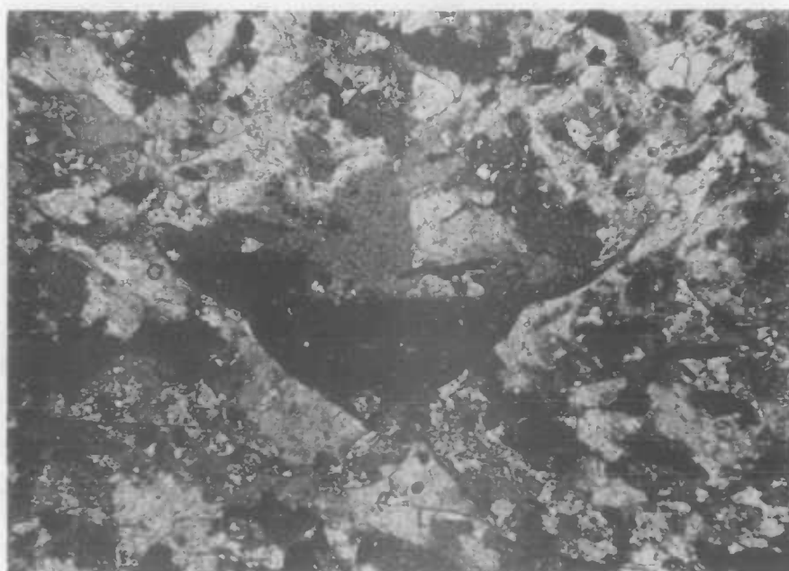
Figure 18: As above, nicols crossed to show isotropic collophane filling and pellets, and the sparry calcite matrix. x 35.
