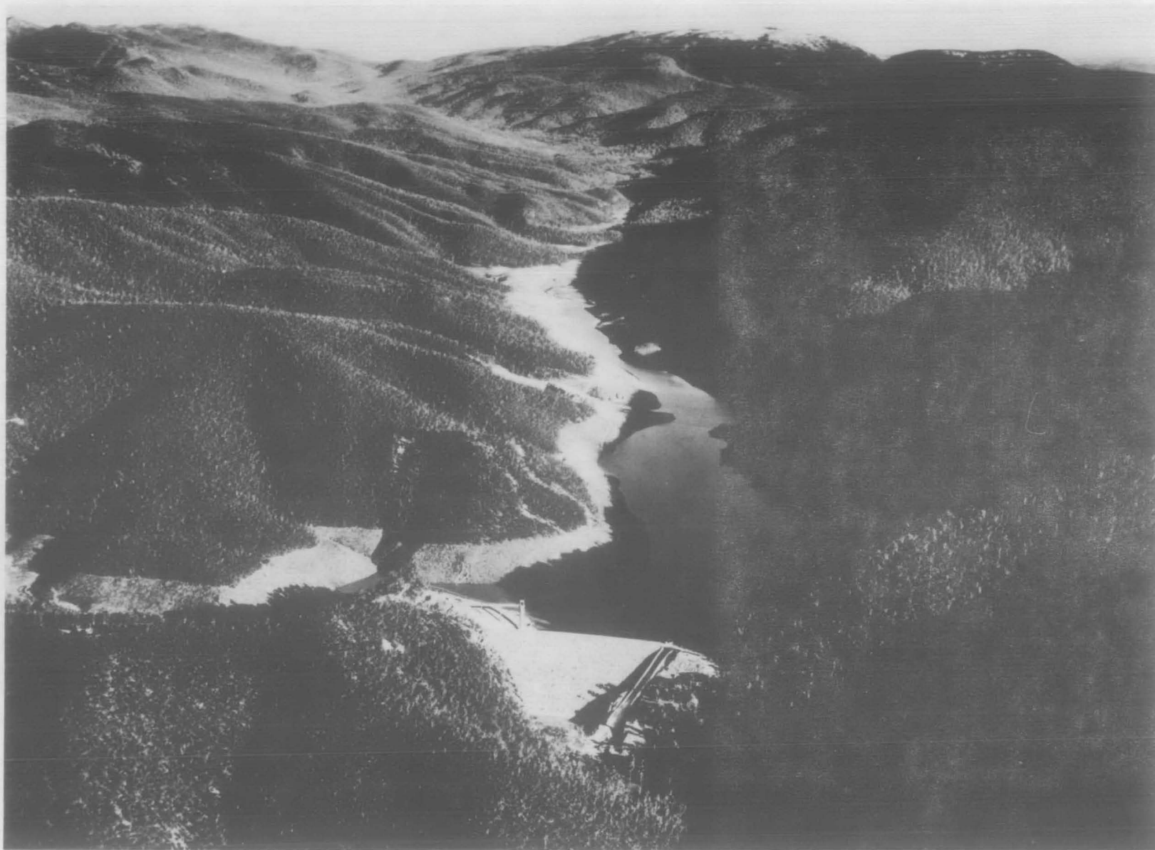
Fig. 5 :- Aerial view of the upper Cotter valley showing Corin Dam and reservoir area 3 months after plugging of the diversion tunnel. Note the subdued topography and gentle slopes in the granite at the head of the catchment area.
