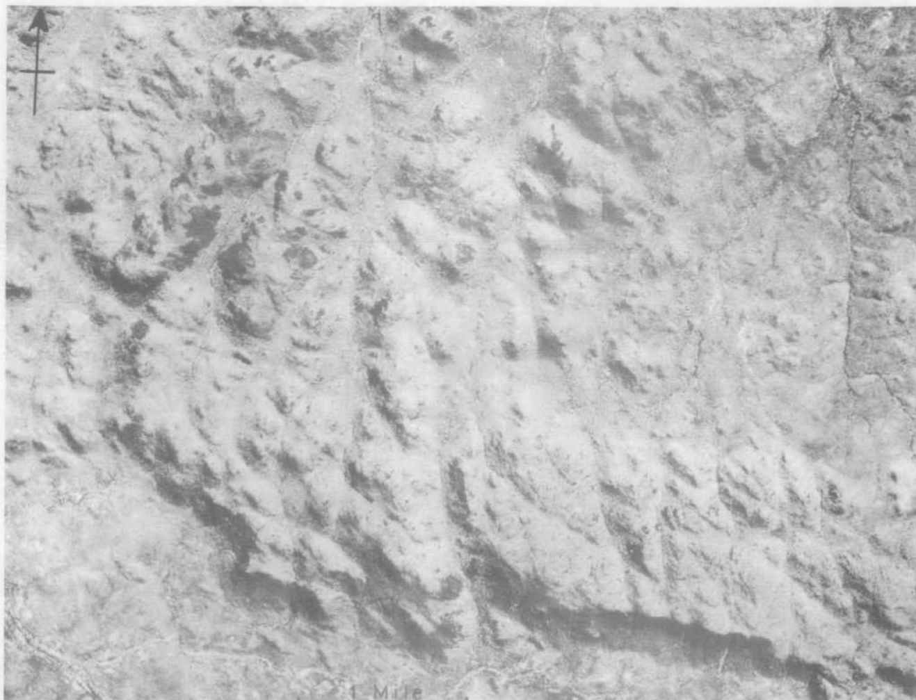
Fig. 2a. Typical physiography of Mondooma Granite. Vertical air photograph. Note black boulder scree and well defined joint pattern. Lennard Granite forms low ground at base of photo. GA 1292 (Photograph by RAAF) Centre point of photograph is 4 miles east-northeast of King Creek Yard.
