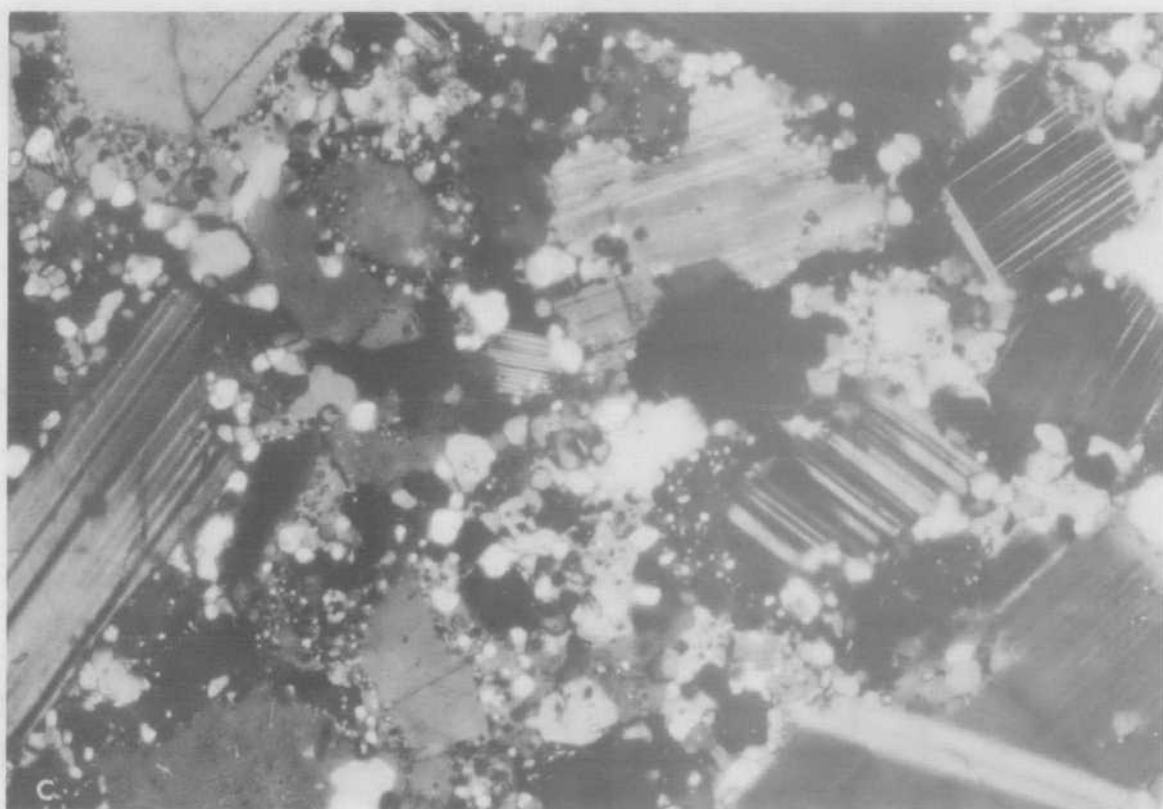
Fig. 12. Textural features of Mendooma Granite (a) Phenocrysts of plagioclase and partly resorbed potash feldspar both containing marginal quartz inclusions; x 28; crossed polarizers. (b) Orthopyroxene bordered by secondary iron oxide; x 28; crossed polarizers. (c) Typical porphyritic Mendooma Granite containing phenocrysts of plagioclase and potash feldspar (with marginal quartz inclusions in a medium-grained equigranular matrix studded with prominent quartz granules. x 36 crossed polarizers.
