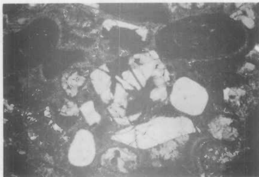
Figure 16. Photomicrograph of calcareous sandstone from the base of the Yalam Limestone shows rounded plagioclase, quartz and lava fragments, and microfossil remains, in calcite cement. Crossed nicols.
