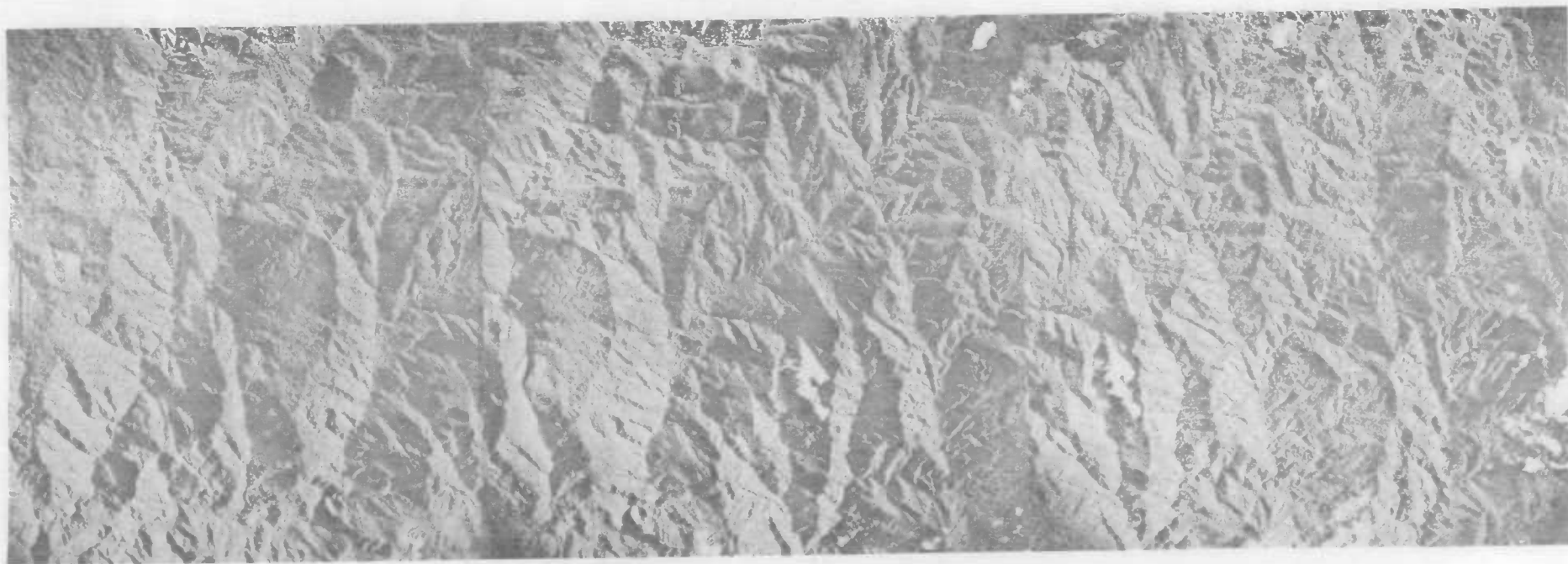
Figure 34. Drainage controlled by faults and joints in the South Baining Mountains (two stereoscopic pairs). Scale 1:100,000 approx.
