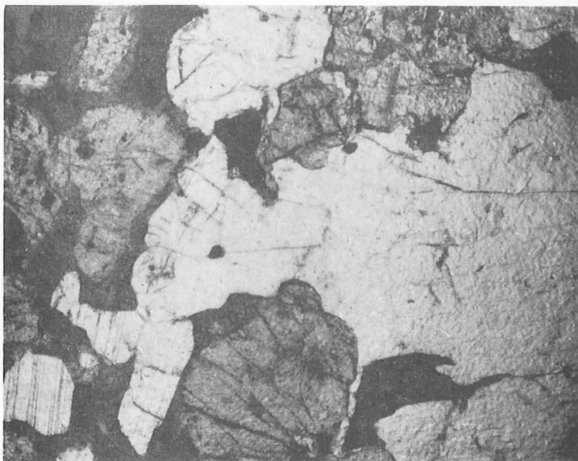
Fig.45 Hornblende-augite gabbro, 2ONG 1270M, from the Bismarck Intrusive Complex, in the Mt. Wilhelm - Mt. Kworu area. Very pale areas are bytownite, light grey augite; darker grey hornblende forms patches in and mantles on augite. Opaque mineral is magnetite. 45X, plane polarized light. Neg. M/1021.
