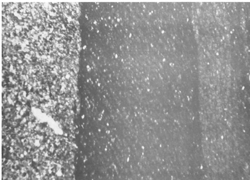
Fig. 11 : Strain slip cleavage at an angle to bedding in finely interbedded slaty shale and siltstone of the Omung Metamorphics. Specimen (21NG0523) from the Kundiawa-Gumine road. X 40, plane polarized light.
