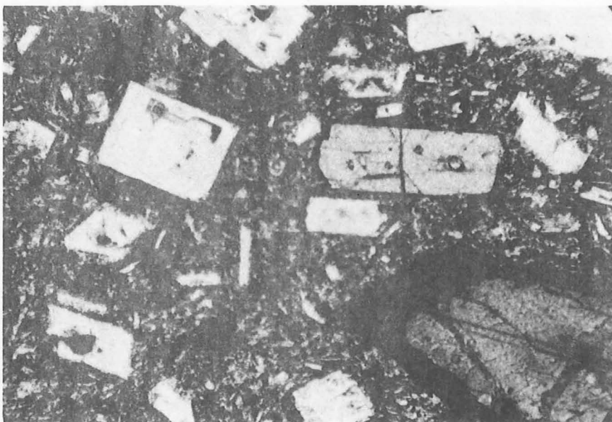
Fig.40 Hornblende-2-pyroxene basalt (21NG4033C) from Crater Mountain. Phenocrysts of labradorite, augite (extreme left), hornblende with magnetite reaction rim (lower right) and hypersthene (upper right) in a groundmass of labradorite, augite and magnetite. 83X, plane polarized light. Neg. M/1021.
