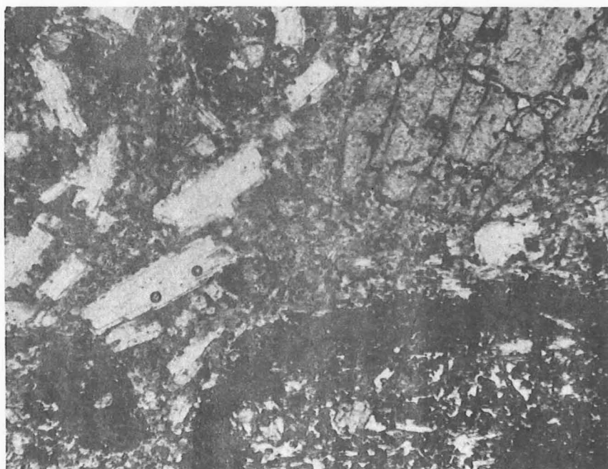
Fig.37 Shoshonite, from Mount Sauru (specimen 21NG 1383C), showing phenocrysts of augite, labradorite, olivine, and hornblende pseudomorphed by pyroxene and magnetite, in a groundmass of labradorite, augite, magnetite and glass. Alkali feldspar forms clear mantles on plagioclase. X83, plane polarized light. Neg. M/1021.
