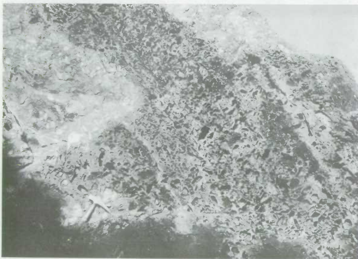
Fig. 34b Hematite conglomerate west end of main ore body, Koolan Island. Pebbles and cobbles of hematite-bearing quartzite are enclosed by a granular hematite matrix. The leached zone consists almost entirely of hematite (Neg. GA 966) DCG
