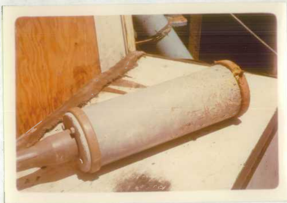
A. Varian magnetometer detector showing shark damage (RV Mahi )
