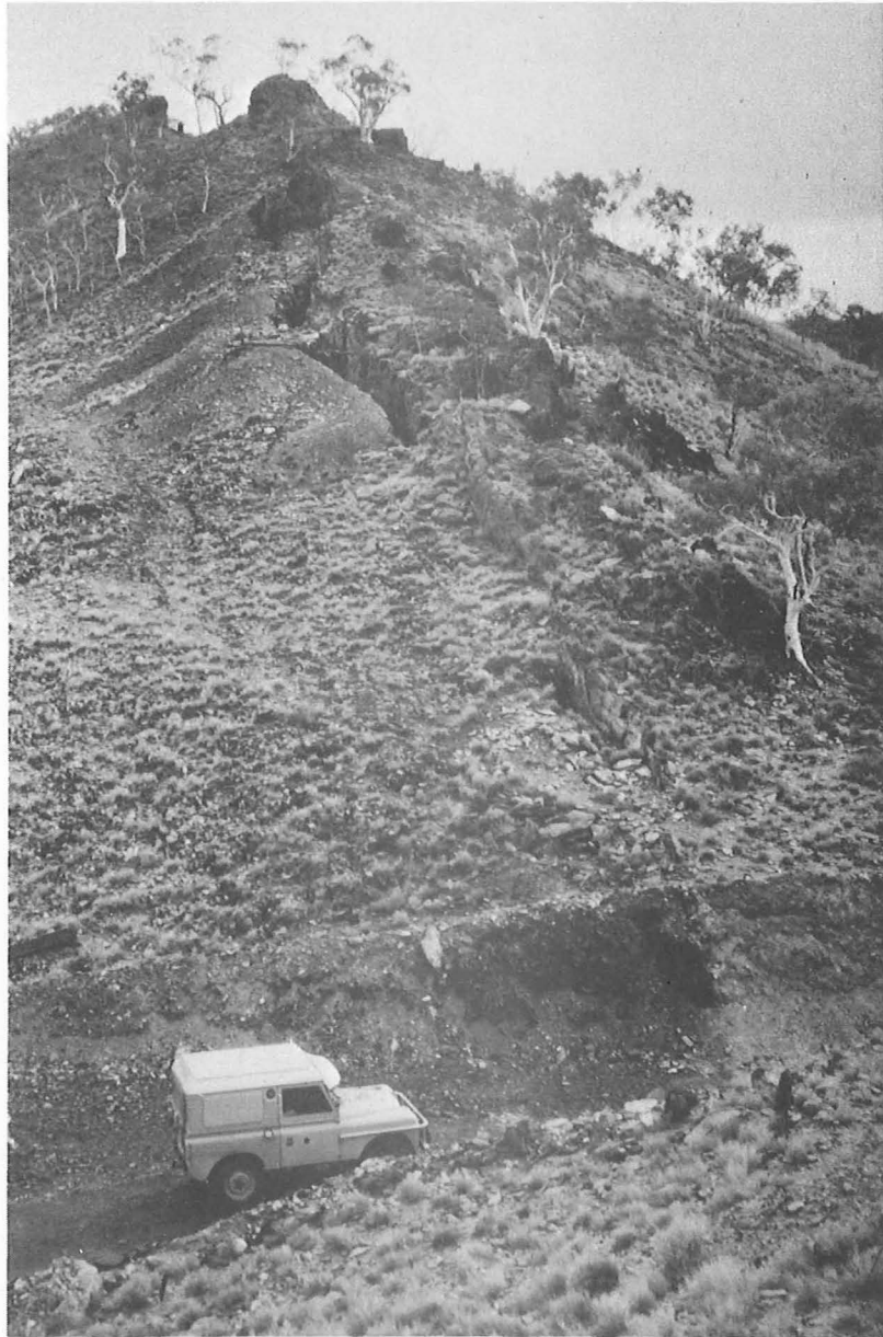
Fig. 107 Lode and workings at Red Sierra South copper mine; hanging wall (right) is bleached and kaolinitic and footwall (left) is black and carbonaceous
