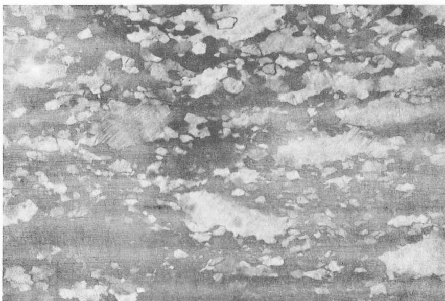
Figure 26. Old, deformed quartz grains with deformation lamellae and new polygonal grains. (Crossed-nicols; spec.loc. 215. Scale as for Figure 22) ANU 579A
