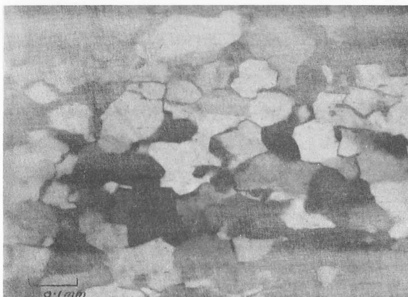
Figure 27. Completely recrystallized polygonal-shaped quartz grains. (Crossed-nicols mag.X136; spec. loc. 279)
