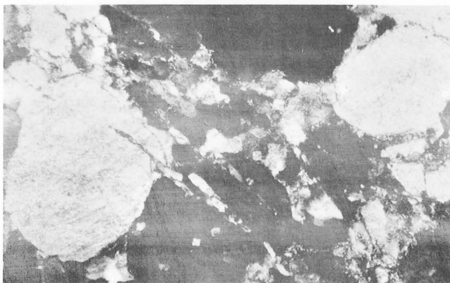
Fig. 44. Photomicrograph of autochthonous Heavitree Quartzite (sp. 281) from 6\frac{1}{2} km south-south-west of White Dam, showing quartz grains with cracks, inclusions, and offsets in fracture zone where recrystallization (small grains) has occurred. Crossed nicols. Length of field = 2 mm.
