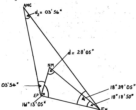
d<sub>1</sub> and d<sub>2</sub> are the corrections to the azimuths observed on Ex to give the required azimuths from EP.
